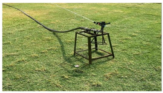
Figure:-Water Sprinkler system in university lawn
